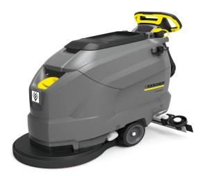
The BD 50/50 C Bp Classic offers a clear view of the area to be cleaned due to the compact dimensions of this battery-powered scrubber drier with sophisticated disc technology. The operation of this machine is as clear as the view with the EASY Operation Panel from Kärcher. Machine features have been reduced to the most important settings and functions to enable use after brief instruction. We recommend the BD 50/50 C Bp Classic for use in supermarkets, hotels or healthcare facilities.
